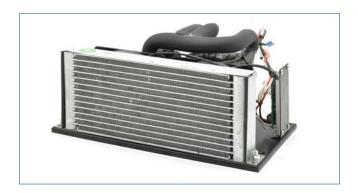
The DC-C coaxial liquid chiller is used to cool drinking water. It has a variable speed compressor driven by 12V /24V / 48V DC power, a high-efficiency micro-channel condenser and a stainless steel coaxial type evaporator.
